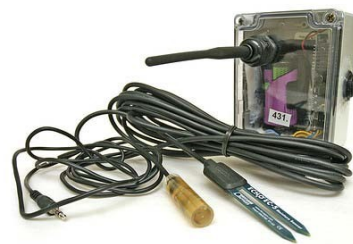
Figure 2: Our Gen-2 platform, based on the Telos mote.
