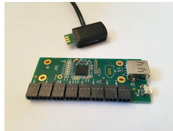
Figure 12: The CC430-based Toast and miniToast analog interface/multiplexer boards.
